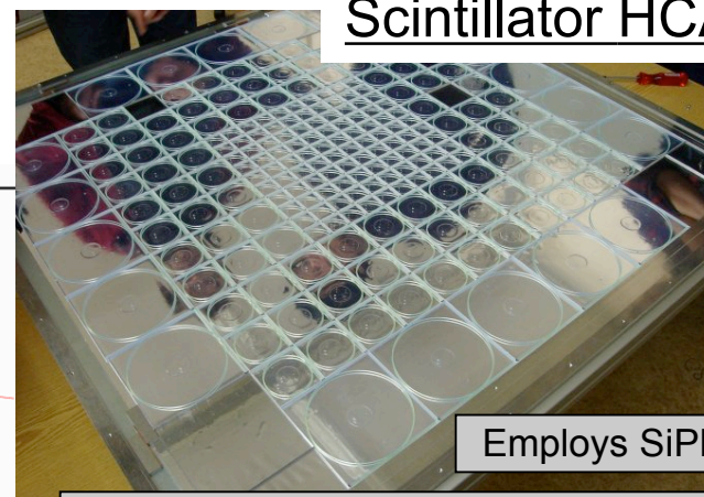
One of 40 layers of the prototype section
